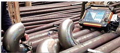
This is used to perform circumferential weld inspections on pipes.
