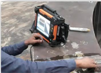
Suitable for flat butt welds inspection.
