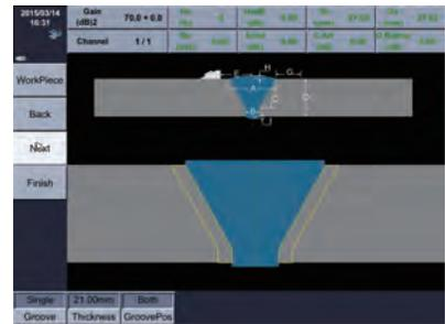
Input weld parameters to set up the workpiece.
