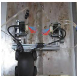
Dual-side Butt Weld Inspection
