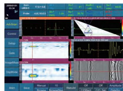
Simultaneous PAUT and TOFD inspection can expand scanning coverage, decrease undetected rate.
