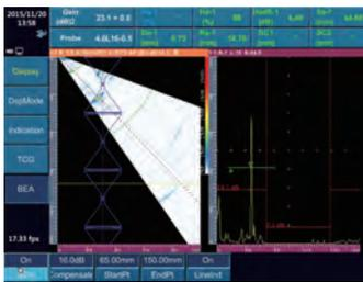
This is to help set a gate over an area and adjust the gain for this area regardless of the global gain. It is very useful for inspection of forgings and castings with allowing independent gain control of the area under the gate with the BEA for backwall echo monitoring.
