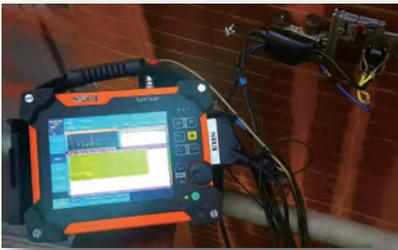
Suitable for detecting loss of wall thickness due to corrosion, abrasion, and erosion on plate and pipe.
